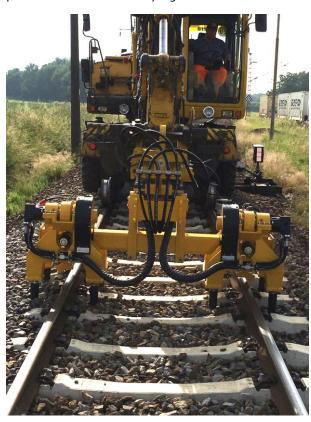
A rotator permits the alignment of the attachment with the sleeper position. All control functions are effected by the operator from the cabin of the two-way excavator.
